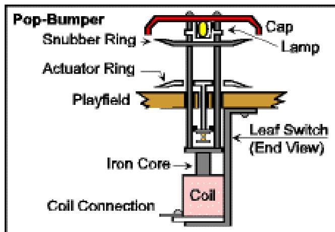
2. When a ball rolls onto the circular plastic actuator, it is pushed down and the central shaft operates the bumper switch. The switch generates an interrupt to inform the computer of its change in status.
