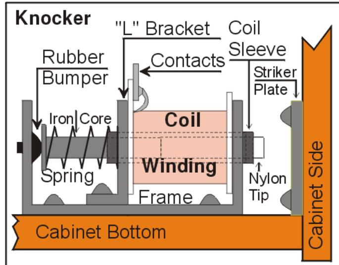
Sometimes the knocker is mounted on the cabinet side and strikes the cabinet base, and sometimes the knocker is mounted in the backbox. The position and direction of the knocker controls how loud a "knock" it makes.
