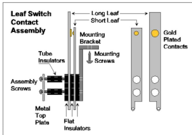
On older electro mechanical machines, two other types of leaf switches may be used. In a normally-closed leaf switch, the longer blade is pushed away from the shorter blade to open the circuit (and turn something off). A single-pole-double-throw (SPDT) leaf switch has a long blade in the center with shorter blades on each side. One side is normally-open and the other is
