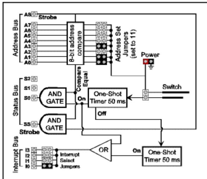
2. If the switch is open when the first one-shot timer expires, the OFF signal from the one-shot timer goes to another one-shot timer. The output of the second one-shot timer is called the *Opened ON* signal.
