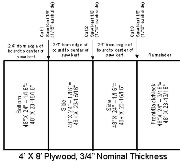
2. Take the front/back/neck piece and make the second set of cuts shown in the diagram. This is done most easily on a panel saw. Usually, the lumberyard will make these cuts at a small cost per cut. The dimensions shown are based on making the cuts at 24" and 16" since each cut takes about 1/16" off of each side for the saw kerf.
