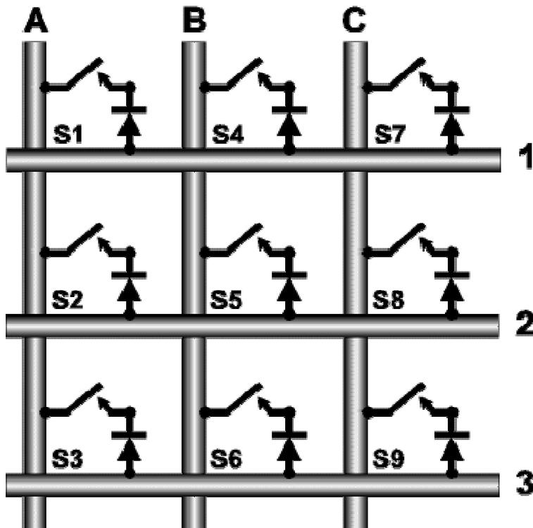
A switch matrix (Fly-by-Wire-1) is used in most modern pinball machines. The picture shows a simplified 3 by 3 matrix. A signal applied to column A gives output for switches S1, S2, and S3 on wires 1, 2, and 3 respectively. Removing the signal from column A and applying it to column B gives output for switches S4, S5, and S6 on the same wires. Similarly, the status of switches S7, S8, and S9 can be read by applying the signal to column C. The diodes at each switch
