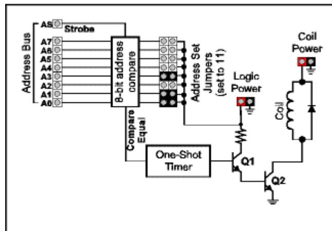
2. The *Compare Equal* signal activates a one-shot timer. The timer in turn activates the coil driver. The timer is used to Images the coil power on long enough to operate the coil, and then shut the power off so that the coil doesn't overheat.
