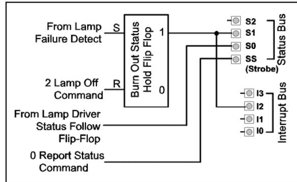
This type of operation is suitable for lamps that have multiple states such as on, off, blinking slowly, and blinking rapidly.
