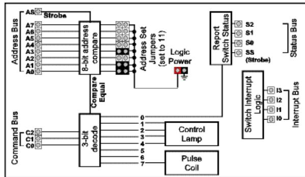
2. When *Compare Equal* is ON, the command decode chip is enabled.
