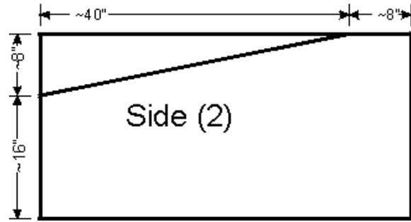
8 inches from the top and 8 inches from the back and draw a line. Cut along the line to create the slope. If you use a power saw, use a clamp-on saw guide to make sure the saw cuts straight.
