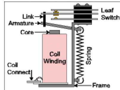
This moves the electrical contacts or switches back to their original position. The total movement of the relay armature is about one-sixteenth of an inch.
