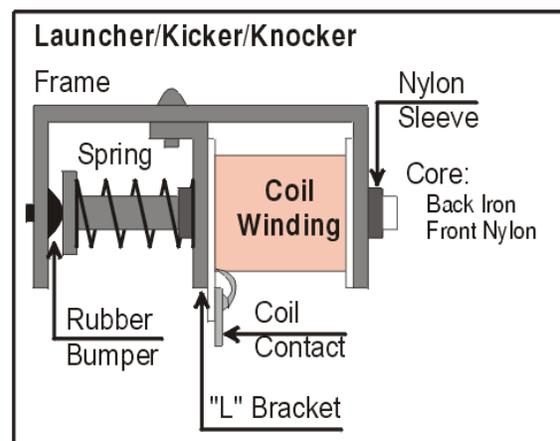
In a pinball game, solenoids are used to provide almost all electrically controlled mechanical motion. Solenoids are used for *flippers, ball launchers, kickers, scoops, drop target reset, bumpers, deflectors,* and various other hidden or public game features.
