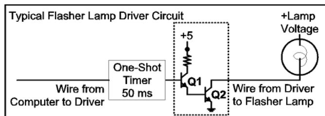
A signal from the computer triggers the one-shot timer. While the timer is running, it turns on low-power transistor Q1 which turns on high-power transistor Q2 causing current to flow in the flasher lamp. The lamp voltage is 2.5 to 4 times the rated voltage for the lamp, causing the lamp to light very quickly and brightly, but the short duration (controlled by the timer) prevents the lamp from burning out from too much power.
