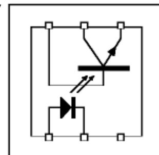
next to each other. Typically, an opto-isolator will be in a small package similar to other integrated circuits.
