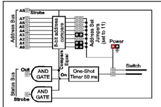
2. When a poll is received on the eight address lines (A0- A7), a strobe is also received on the Address Strobe line (AS) to indicate that the address is stable and ready. The *Address Strobe* signal enables the eight-bit comparator. The address lines are compared to the signals from the eight jumpers. If both are the same, the *Compare Equal* is set ON.
