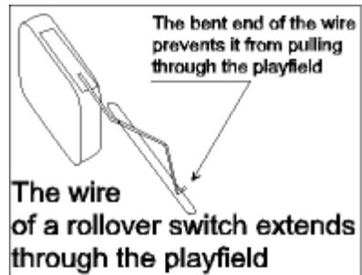
Microswitches with wire actuators are used for playfield roll-overs. The wire is bent to stick up through a slot in the playfield. When the ball rolls over the wire, it pushes down on the wire which operates the switch. Microswitches with blade actuators are used for detecting a ball passing through a gate. As the ball moves the wire gate, one end of the wire swivels down to press the blade which operates the switch.
