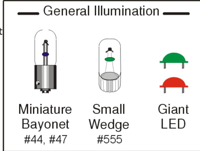
General illumination lamps are not individually controllable. The whole string of lamps is controlled by a single relay. (There may be more than one string of general illumination lamps.) Because they are not individually controllable, they do not require diodes and can run on AC power. An entire string of general illumination lamps only requires two wires for all of the lamps. General illumination lamps are cheap.
