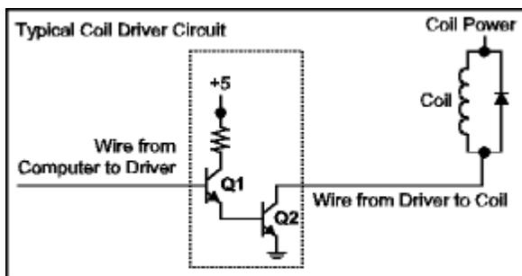
A signal from the computer turns on low-power transistor Q1 which turns on high-power transistor Q2 causing current to flow in the coil. The diode across the coil routes the high-voltage spike, generated by the sudden collapse of the magnetic field when the coil is turned off, back into the coil instead of into the circuitry.
