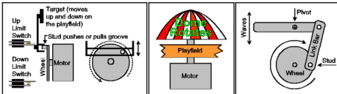
Motors are used in pinball machines with many variations of mechanical linkages. A motor can cause rotation of a dome, a back and forth or up and down motion, and many other variations. A motor with "limit" switches is used to control features that rise from below the playfield, stay in play for a while, and then disappear below the playfield again.
