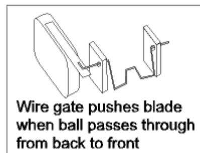
Microswitches are used on both electro mechanical and modern pinball machines. On modern machines, they carry low voltages and very small currents, so they are very reliable.
