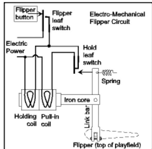
4. The holding coil holds the iron core so that the flipper remains in the up position. The holding coil uses less electricity and generates less heat than the pull-in coil. It is strong enough to hold the iron core in, but is not strong enough to pull the iron core in by itself.
