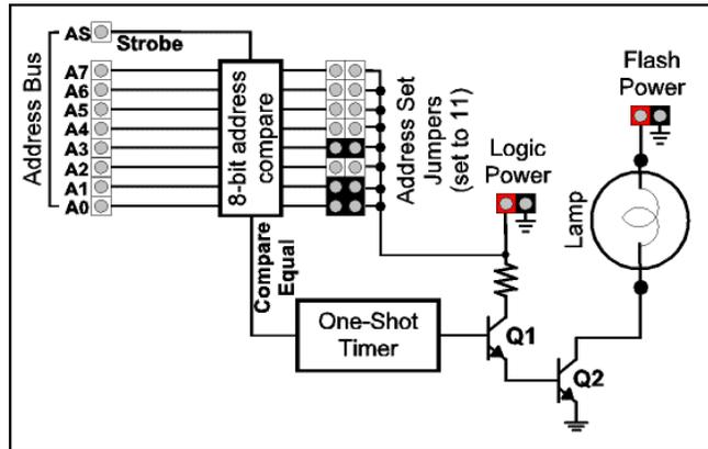
2. The *Compare Equal* signal activates a one-shot timer. The timer in turn activates the lamp driver. The timer is used to Images the lamp power on long enough to flash the lamp, and then shut the power off so that the lamp doesn't overheat and burn out.
